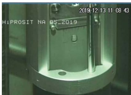
Post-irradiation underwater visual inspection of a FUTURE-5 fuel plate
